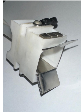
Fig. 10. 3D Printed GFPPT-I. Following the CAD design and specifications, three permanent magnets were inserted in the front most dedicated space. Stainless steel was utilized on the parallel electrodes, with a 45° flap, and steel screws were utilized to attach the high-voltage feed cables, as well to act as a high-voltage electrode.
